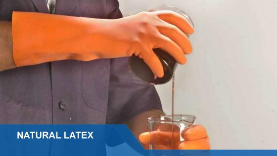
Natural rubber or natural latex is flexible and soft, yet tough and durable. It is used to make both supported and unsupported gloves which offer economical solutions to a wide range of chemical hazards.
